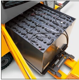
Sideways battery removal
